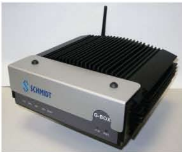
興華科儀的G-BOX是一部綜合式的無線射頻識別(RFID)讀寫器。 G-BOX is an all-in-one industrial grade RFID reader self-developed by Schmidt.
