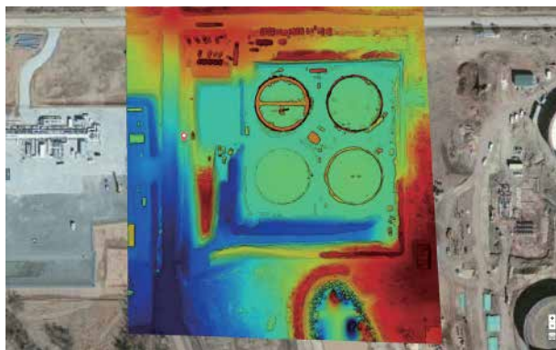
A highly detailed drone-captured orthomosaic map of a construction project in the U.S., overlaid on the background satellite map.
