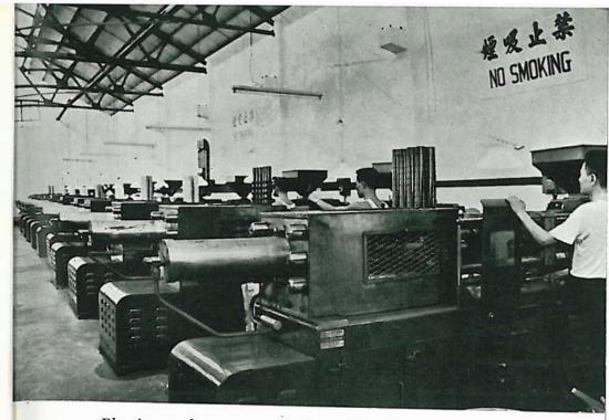
Plastic goods are one of Hong Kong's most important exports. Above, a bank of locally made injection moulding machines: below, a mould in the making.
